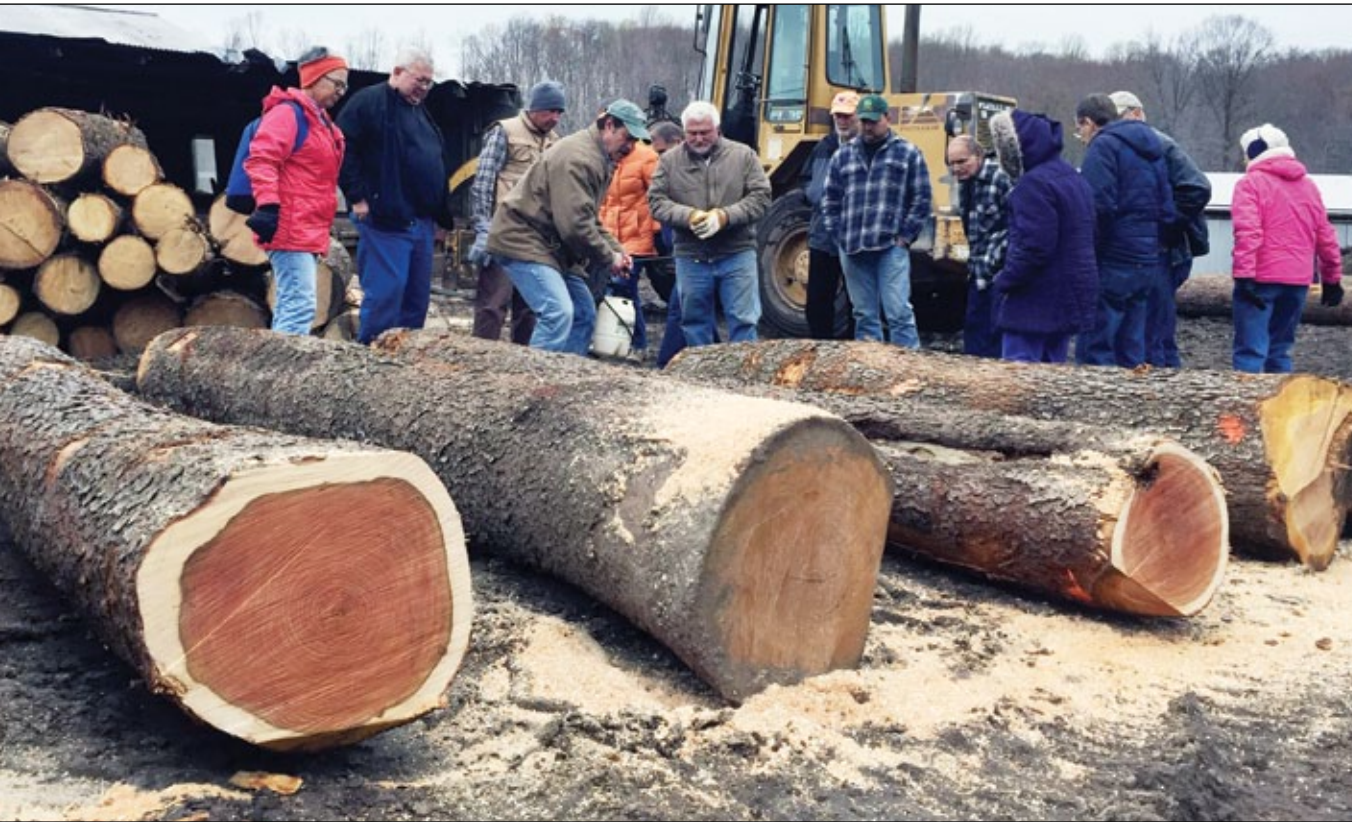
On a field trip to Champion Lumber Company, Champion, our forester (center) showed participants how to evaluate the bottom end of a potential veneer log for defects.
