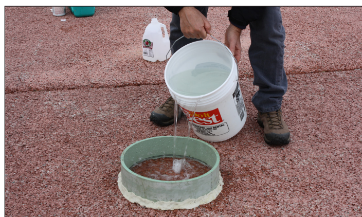
Testing the infiltration rate of permeable paving using ASTM 1701 test standards.
