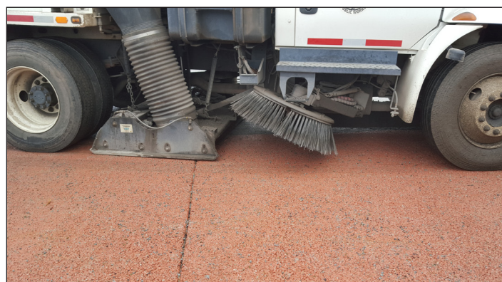
Vacuum truck on permeable concrete
