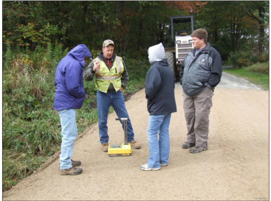
Attendees learning about the importance of proper compaction and moisture in DSA placement using a Nuclear Density Meter
