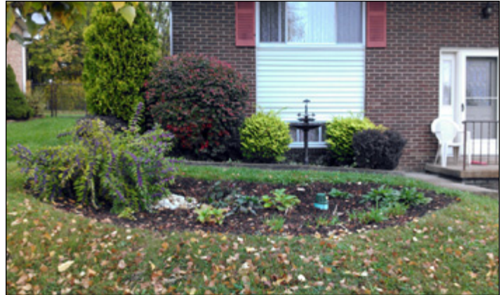
A residential rain garden can be integrated into a landscape to capture and treat roof runoff.
