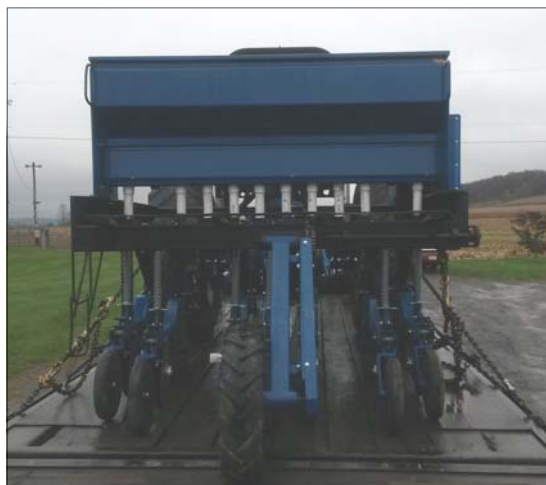
Farmers and researchers have been experimenting planting a cover crop between crop rows (such as field corn or sweet corn) while the crop is approximately "knee high." One piece of equipment that was tried in Snyder County was an interseeder (above), a no-till drill designed to plant between row crops spaced 30 inches apart. Farmers walk through an unharvested corn field where the interseeder was used during a Conservation District field day event (left). Notice the established cover crop between the corn rows (left and below).
