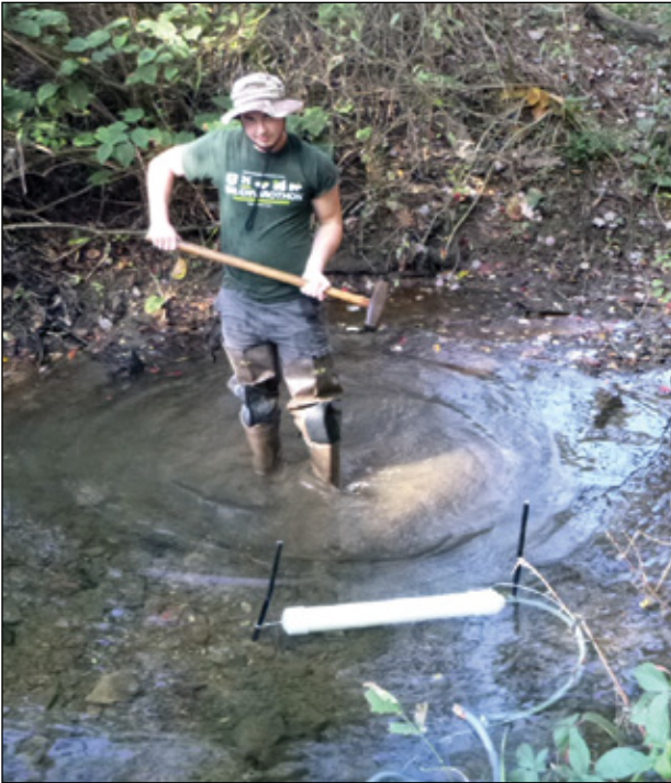
A water-level sensor and a rain gauge were installed near Four Mile Run in a partnership with Saint Vincent College.
