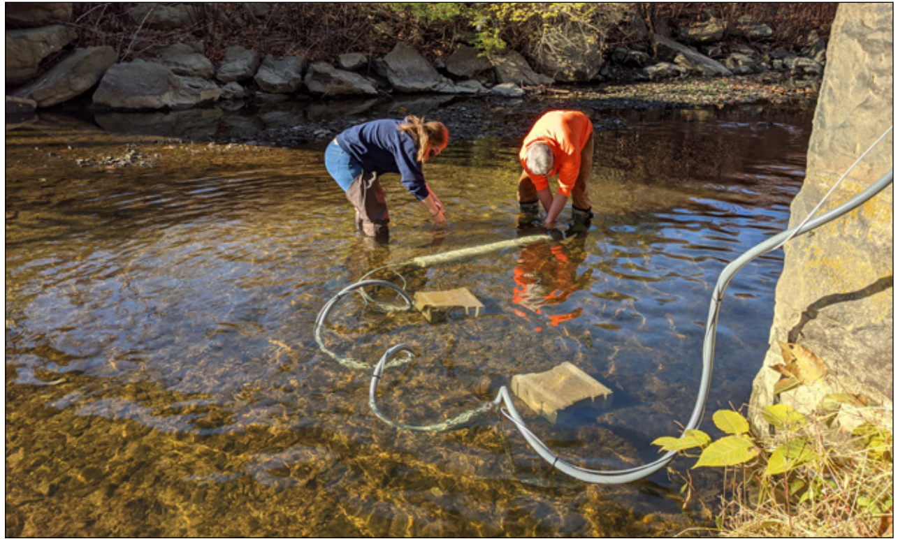
Our watershed technician and a volunteer associate board member installed a data logger to monitor the water quality in Turtle Creek.
