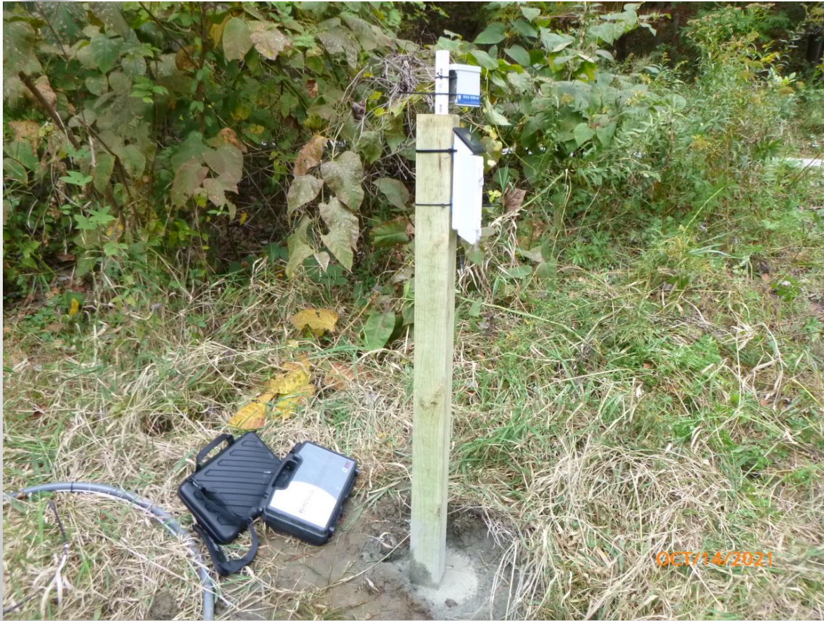
4x4x6 Post, 50lb bag of concrete mix, & a multitude of zip ties
