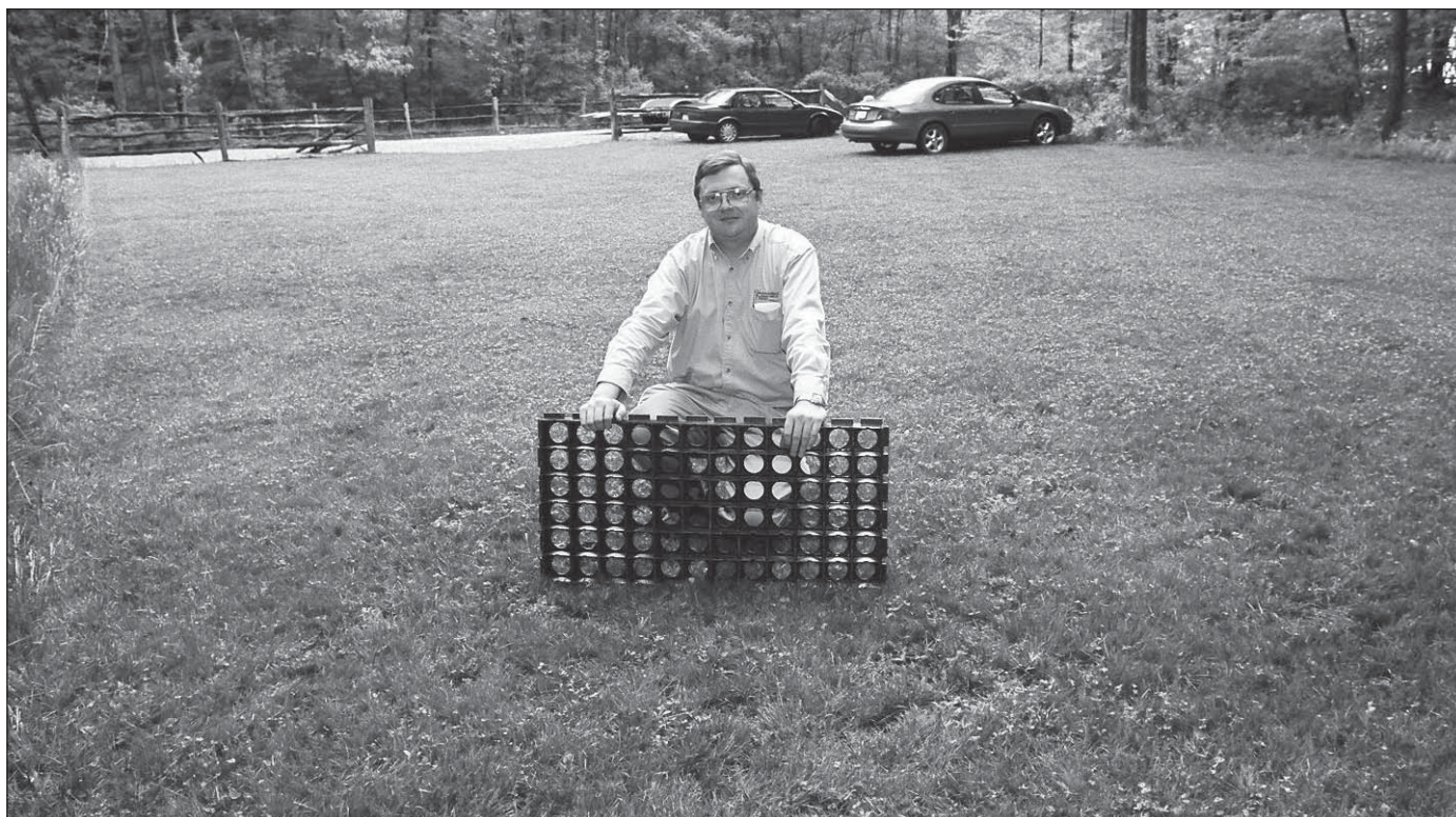
Jim Pillsbury, Westmoreland Conservation District hydraulic engineer, holds a sample of the plastic grid that is installed under the grass to help stabilize this infiltration parking lot.
