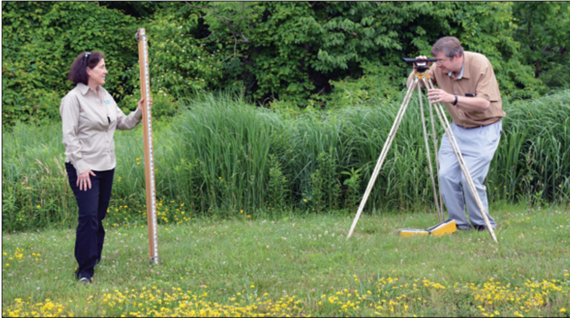
In the field, stormwater staff members Kathy Hamilton, landscape architect/stormwater technician, and Jim Pillsbury, hydraulic engineer, use equipment to verify that stormwater best management practices are built according to plan specifications while Stormwater Technician/Landscape Designer Matt Zambelli runs computer models of proposed stormwater practices.
