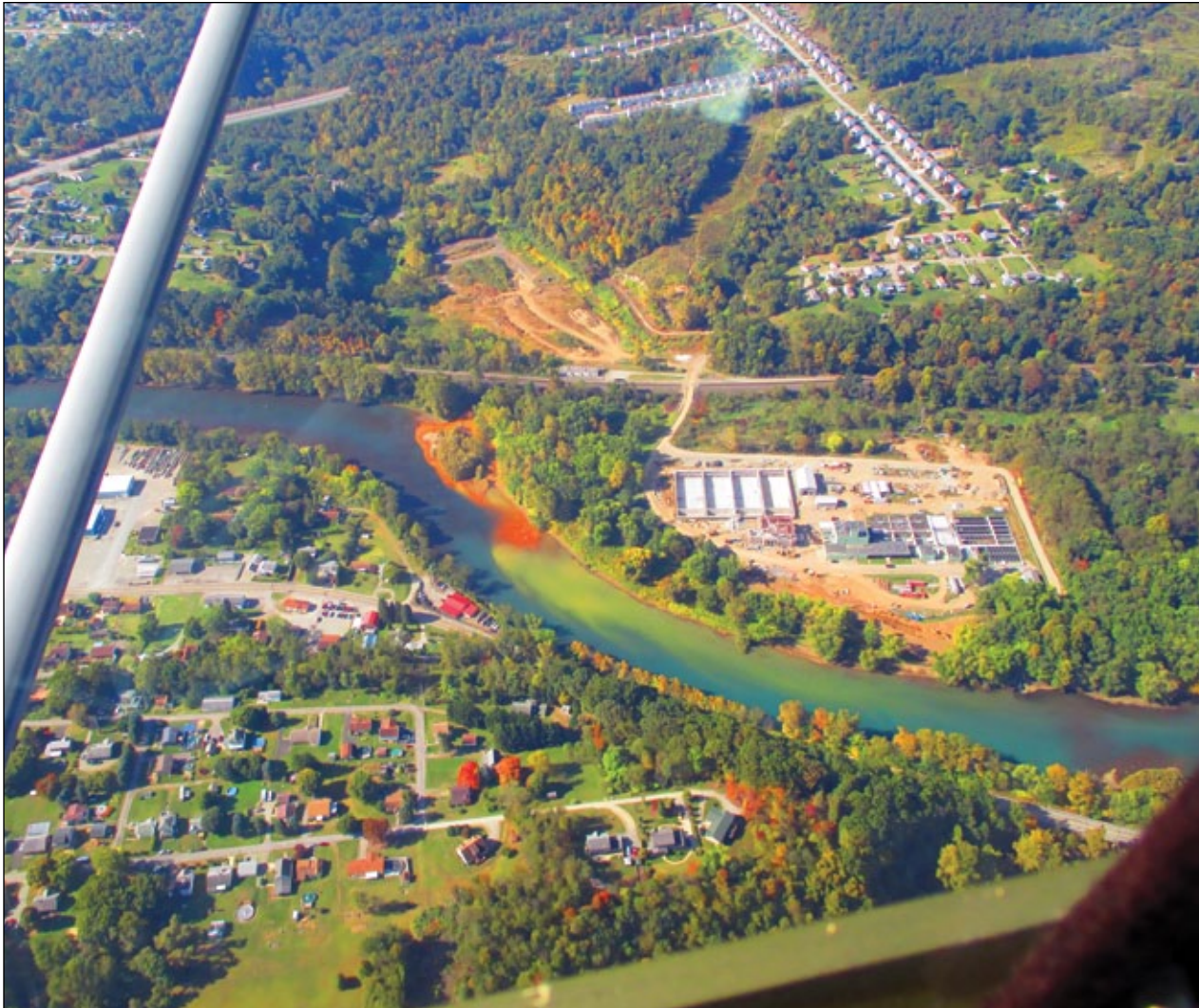
Aerial view of the confluence of Pine Run and the Kiskiminetas River, showing the orange plume of abandoned mine drainage. The sewage treatment plant is just to the right of the plume.
