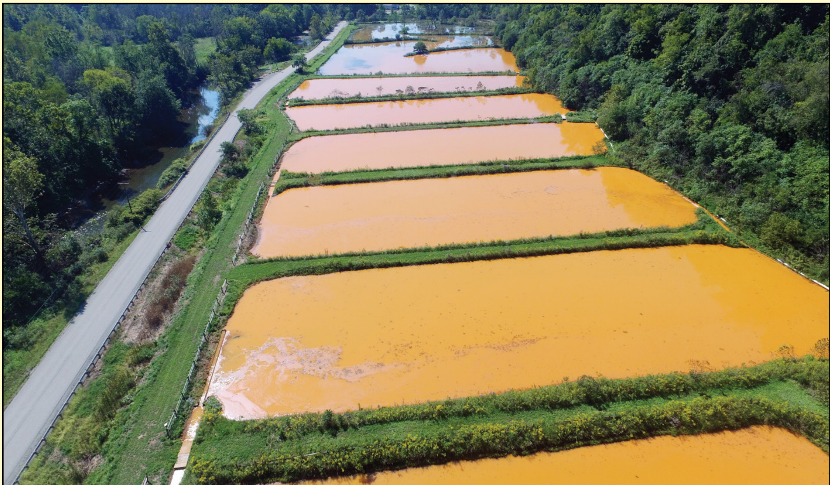
At the Lowber passive abandoned mine drainage treatment system, mine water travels through a series of ponds so iron oxide can settle and filter out before the water enters the Sewickley Creek ( top left ). This site offers various public education opportunities including interpretive signs, special programs and a scenic walking trail.
