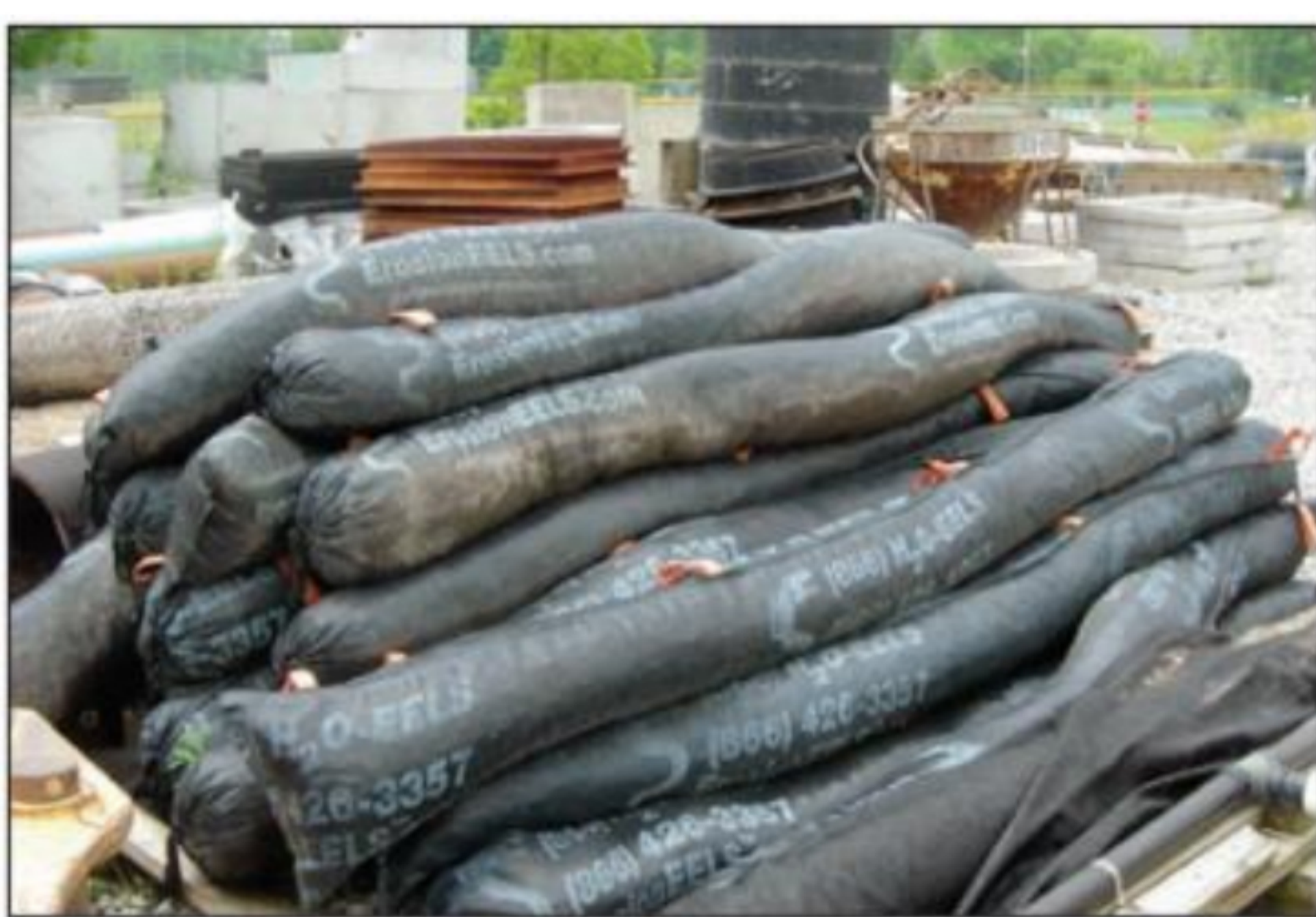
Filter tubes ready to be used on a site. Undamaged tubes can be reused.
