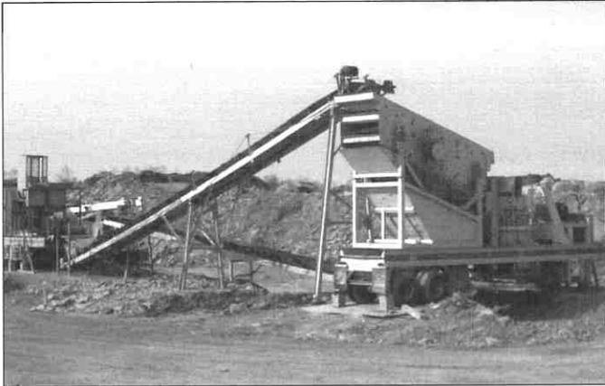
Giant rock crushers break down the giant rock un-earthed to create rock for stable fills.
