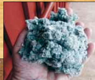
One of the insulations used is made out of recycled newspapers.
