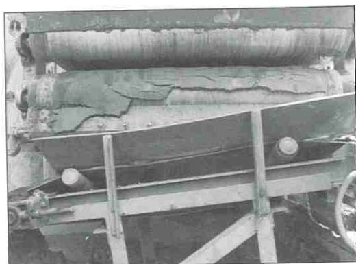
The iron oxide is dried and compressed so that it can be used to manufacture pigment.
