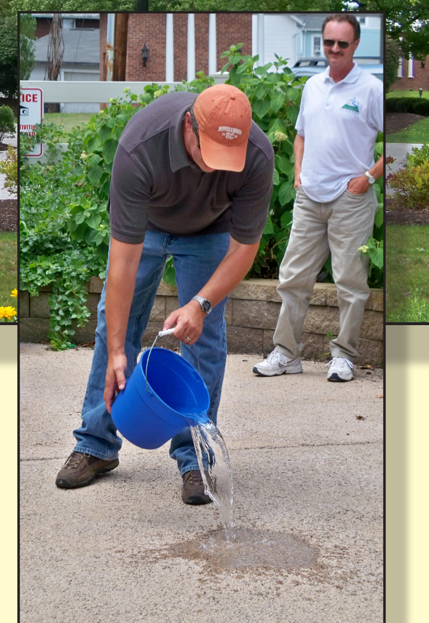
Scottdale's Gazebo Park now features porous pavement, a special material that allows rain to pass through and be absorbed into the ground.
