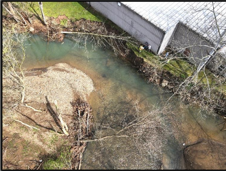
Before: Streambank erosion threatening the building.
